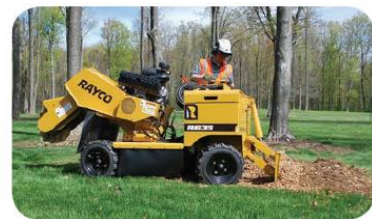
Wide Tires Increase Traction and Floatation
