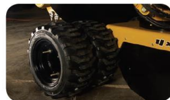
Dual Rear Wheels for Increased Stability and Traction
