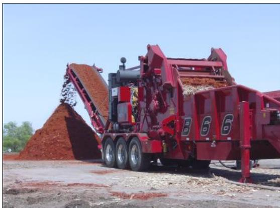
The B-66 can be equipped with the optional Rotochopper patented grind and color system for making perfect colored mulch in one pass.
