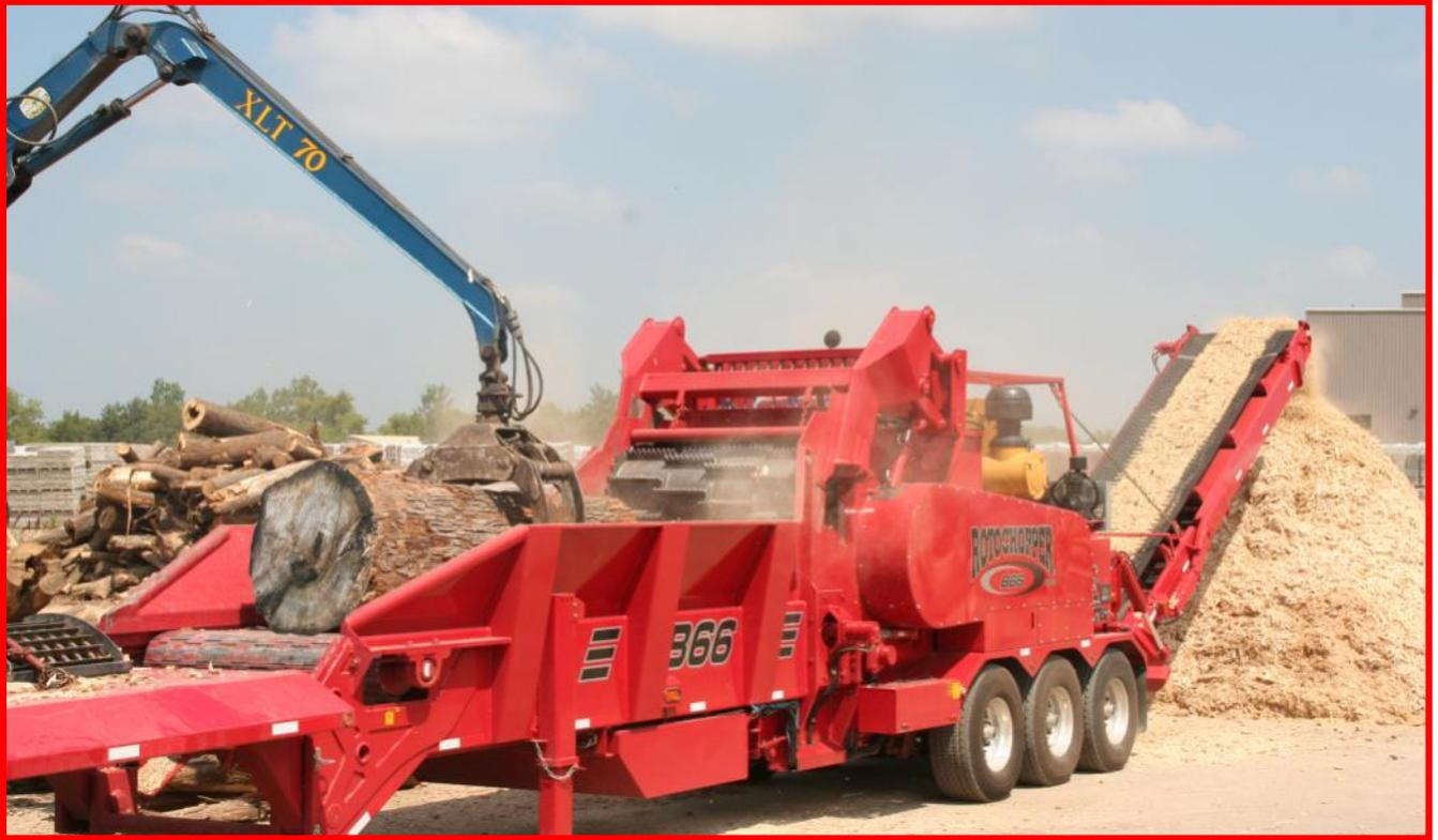
**Diesel or Electric Horizontal Grinder**
