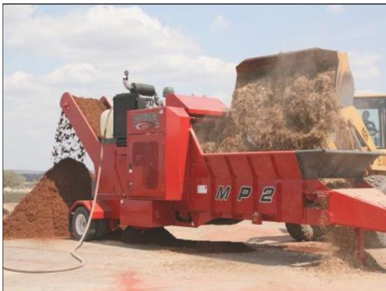
The MP2 comes standard with the patented Rotochopper grind and color system for making perfect colored mulch in one pass.
