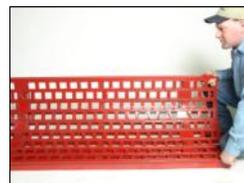
Part of the famous **Perfect In One Pass™** Rotochopper finished product quality is due to our unique screen design. Along with precisely engineered baffles, the shape, location, and relationship of the screen to the rotor are all designed to produce near perfect uniformity in finished product. All Rotochopper models employ a simple one piece screen design. Made
