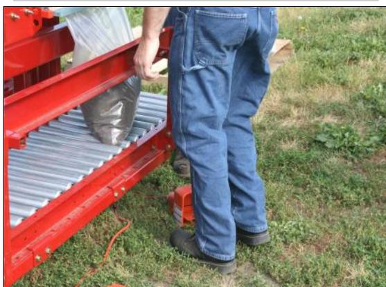
Easy to use foot pedal controls operate the bagging jaws and sealer.
